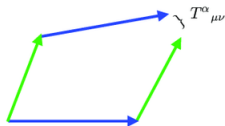
The non-closure of parallelograms formed when two vectors are transported along each other is given by the torsion: Teleparallel Equivalent of General Relativity.
