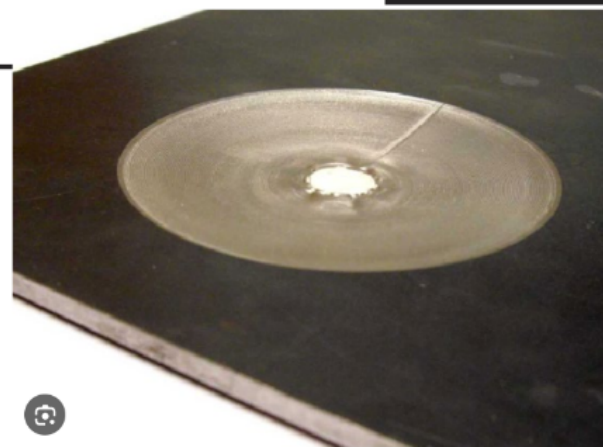
View of a manufactured two-dimensional acoustic black hole embedded... | Download Scientific Diagram
