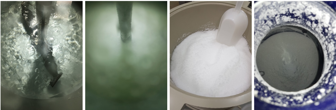
Boiling of solution Recrystallized crystals and mother solution Filtration and washing the crystals Dry the crystals in the conical dryer
