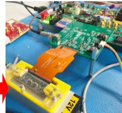
Module testing (Alvin Readout system developed at IFAE)
