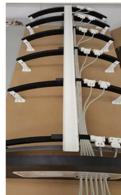
Real size mock-up to check envelopes and train connection of services
