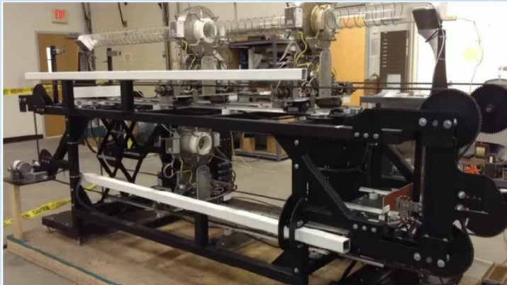
zone refiner suitable for ~100 kg crystal production
