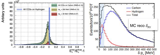
Target material is CH => selecting events with small δpt will allow to select interactions with small nuclear effects or H
