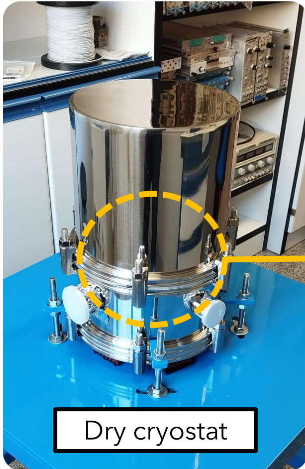
Cryocooler + He Compressor Capability to reach T < 30 K.
