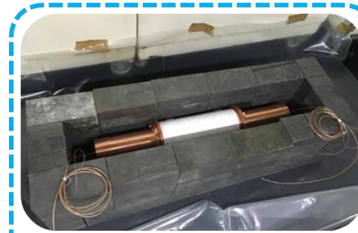
Blank module: same structure as ANAIS module, but without the NaI(Tl) crystal → used to study the PMTs noise events.
