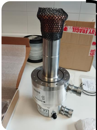
Cryocooler + He Compressor Capability to reach T < 30 K.
