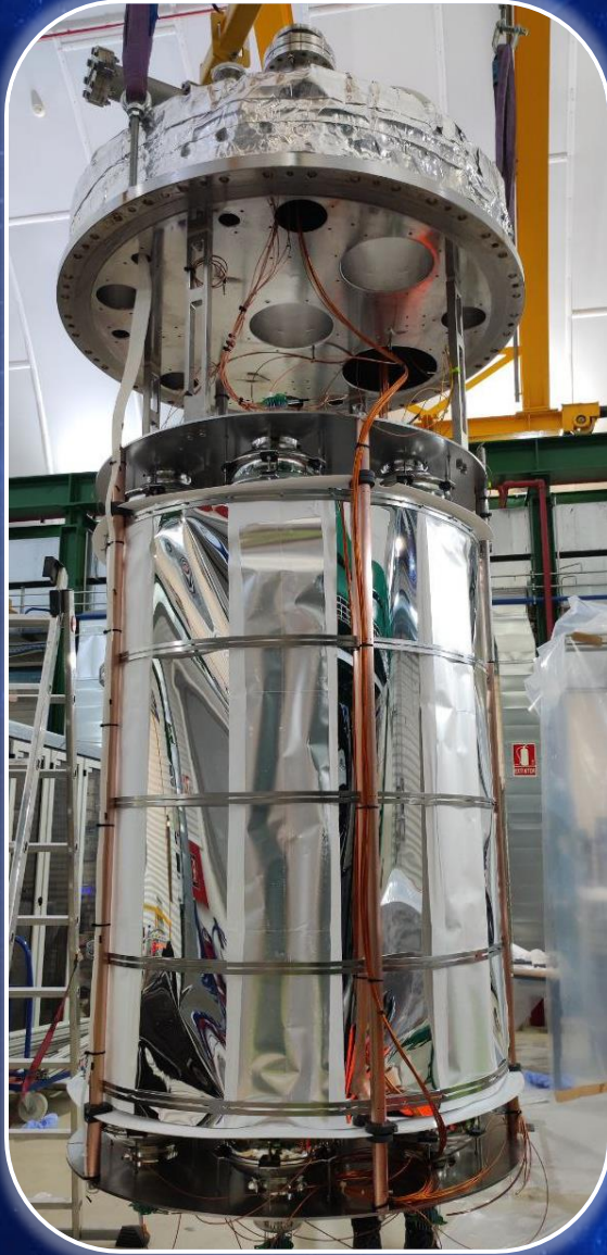
Reflector Coated with TPB
