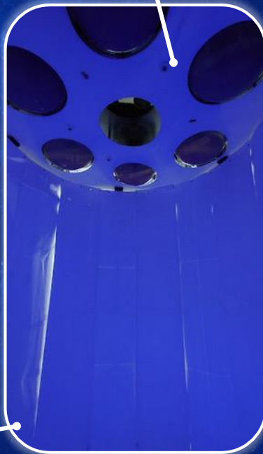
PMT Plane with reflector coated with TPB
