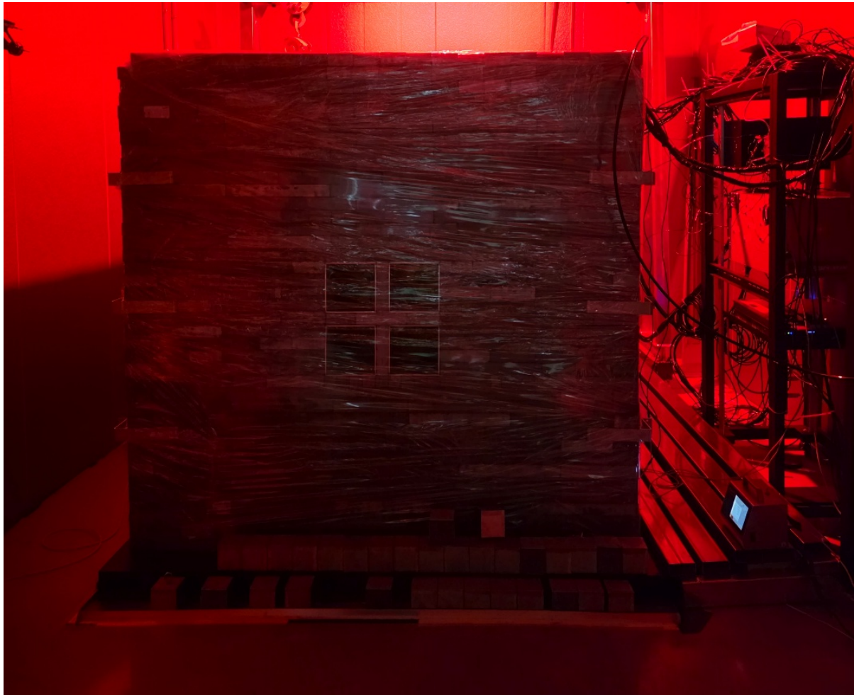
Wrapping the shield to prevent air contamination
