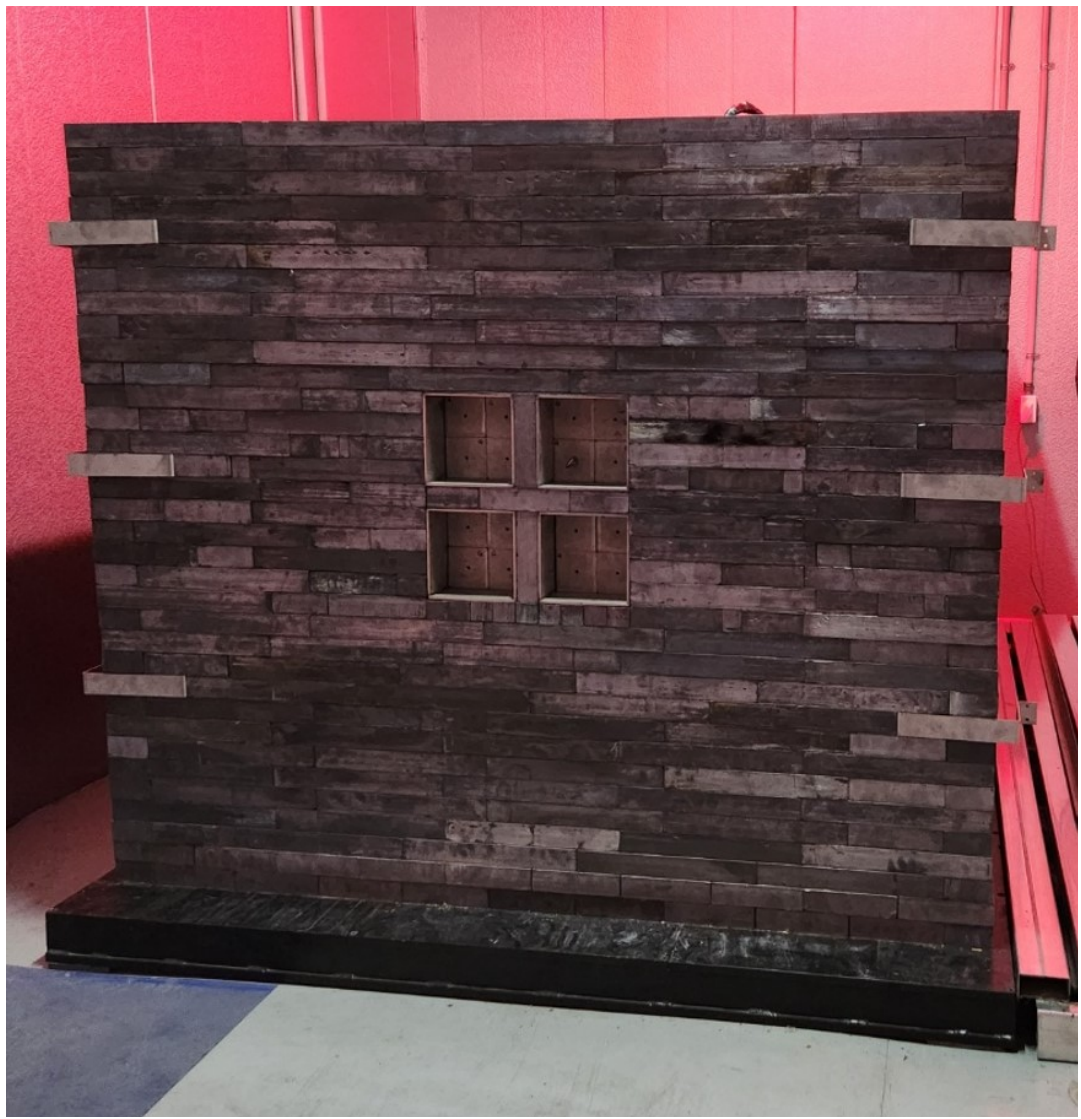
Install side lead shield
