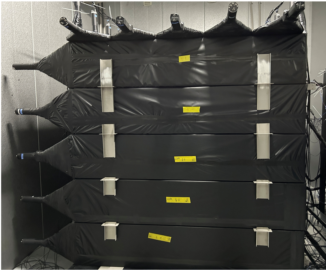
Install Plastic scintillator for muon veto
