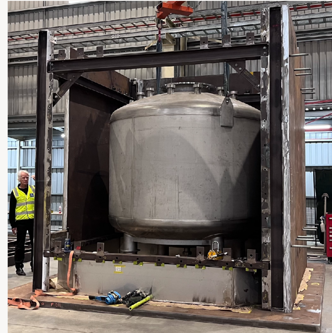
Test assembly of steel shielding and vessel fit-test
